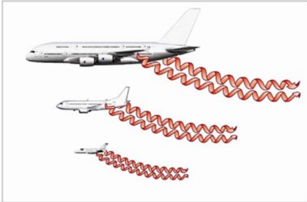
Figure 5 Wake vortices versus aircraft size
